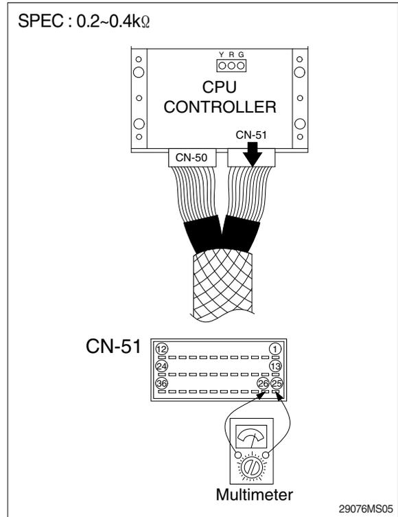
(4) **Test 8** : Check resistance at speed sensor.
