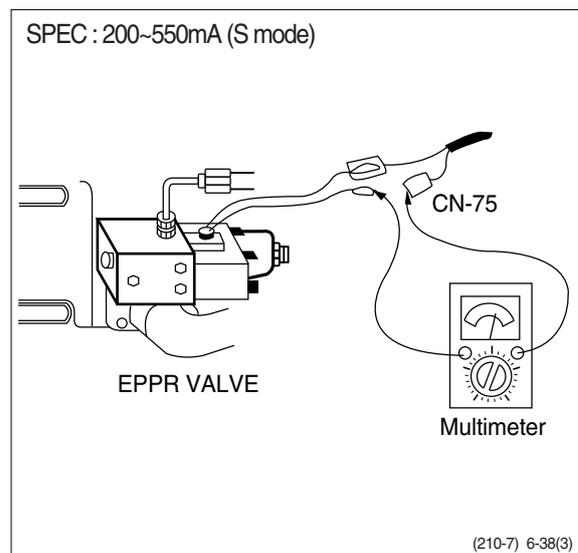
(2) **Test 4** : Check pressure at EPPR valve.
