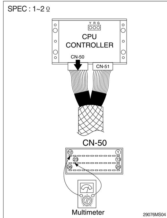
(2) **Test 6** : Check tachometer(Work properly or not)
